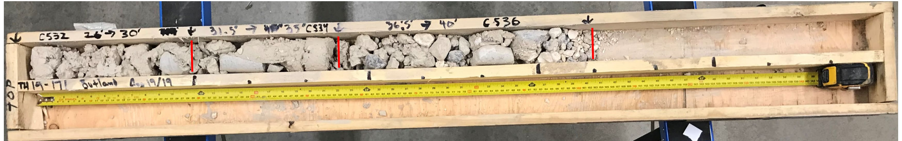
C532) Core Depth: 26 – 30 ft (7.9 – 9.1 m) - 25% recovery C534) Core Depth: 31.5 – 35 ft (9.5 – 10.7 m) - 24% recovery C536) Core Depth: 36.5 – 40 ft (11.1 – 12.2 m) - 40% recovery
